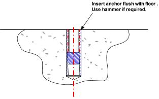
7. Tap anchors into drilled holes using hammer or mallet. When top of anchor is flush with mounting surface, use setter rod to expand and secure.
